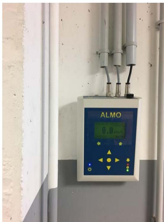
FIG. 30. An area radiation monitor placed at the entrance to or exit from the treatment area to detect a low dose rate source, or an animal with a source, leaving the room or the controlled area. The area radiation monitor can also be used to confirm that a high dose rate source is back in its 'in-safe' position inside the afterloading unit (in the room). (Courtesy of Vetotech, Villeneuve d'Ascq.)
